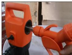
2. Place the Nozzle into the receiving container to transfer the liquid.
