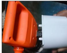
2. Push a fully charged battery into the Battery holder.
