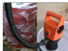
5. Place the Nozzle back into the Holster to prevent any damage to the Hose or to the Nozzle.
