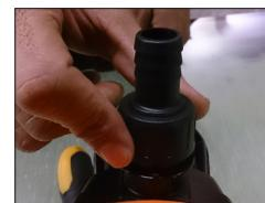
2. Unscrew all the bolts to Remove the Hose Barb from the Outlet.
