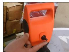
4. After Dispensing Switch Off the Toggle switch (Down) and lift the Nozzle upward allowing all the liquid in the line to flow back into the Drum.
