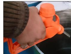
3. Switch On the Toggle switch (Up) and pull the Nozzle Trigger.
