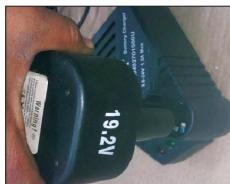
**Note:** Press the side buttons on the battery while removing it or it will not come out.
