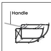
4. Insert Handle into slot to pick up drum make sure that the hook on the handle goes at the top
