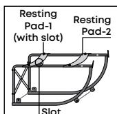
3. Attach Cross Leaf onto the Frame by using 5 nuts & bolts (1 small for the center and 4 medium for the sides).
