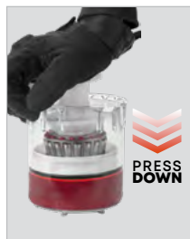
Press the cap until the old grease is forced out and new grease shows on the bearing
