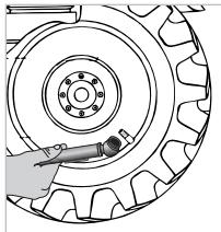
Mate the mouth of the tyre pressure gauge with the air valve of the tyre
