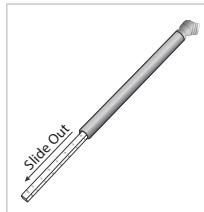
Check the reading on the pressure reading tube that slides out of the tyre pressure gauge
