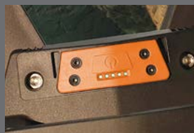
Battery Level Indication on battery pack via 5 LED battery level indicator. Each Led indicates 20% charge
