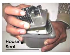
6. Rotate & reinstall Counter Assembly (7) in the desired position. The display can be chosen from one of the following positions.
