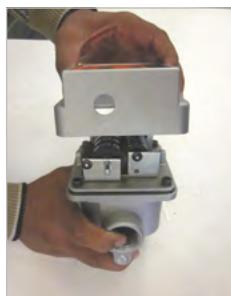
3. Unscrew the four Allen bolts (6) anticlockwise with allen key (size 4).
