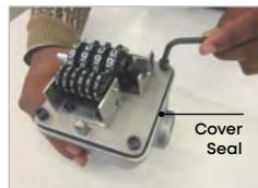
5. Remove Counter Assembly (7) taking care not to damage the Housing Seal (13).
