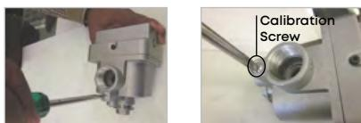
**NOTE:** Always fix the Calibration Screw with O-Ring (15) to avoid leakage.
