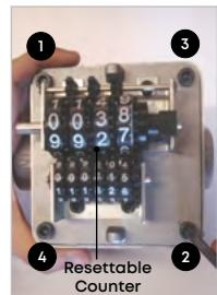
**NOTE:** After installation, rotate the resettable counter with fingers & ensure their smooth movement.
