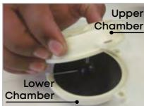
4. Use a soft brush to clean the Measuring Chamber (14). Be careful not to damage the plastic components.
