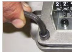
4. Carefully remove the Cover Seal (5).
