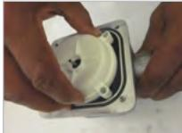
3. Remove O-Ring (10) and disconnect Upper Chamber (9), Lower Chamber (12) & Nutating Disk (11).
