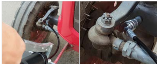
Convenient access into narrow, inaccessible greasing joints
