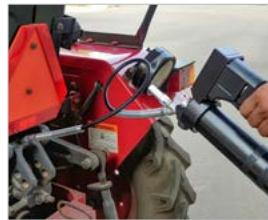
Without Swivel - Twisting of hose
