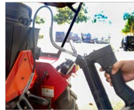
With Swivel - No Twisting of hose
