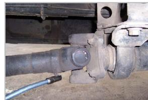
Right angled coupler used for greasing the axle of a low height truck where access to the grease fittings is only through a side
