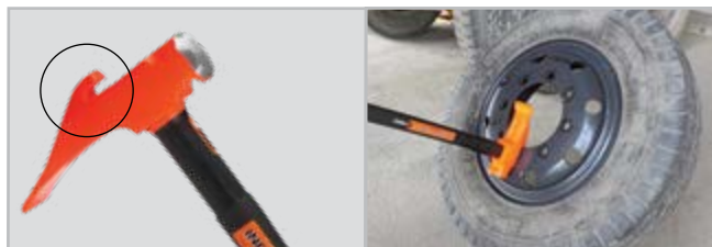
Top Hook used to tip wheel to change sides
