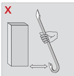
Regular wrecking bar claw angle prevents use near flat surfaces
