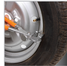
Pliers being used to detach wheel balancing weights
