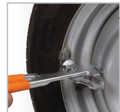
Hammer end being used to form wheel balancing weights
