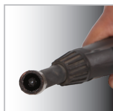
Welding Gun Nozzle filled with weld splatter
