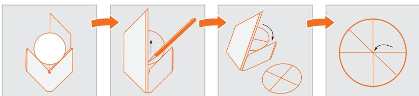
Position the Center Square Vee's on the round stock near the end face
