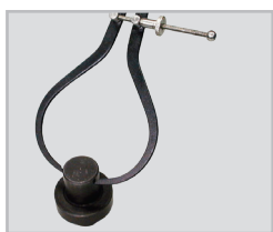
Outside Caliper: Used to inspect the external diameter of a machined component
