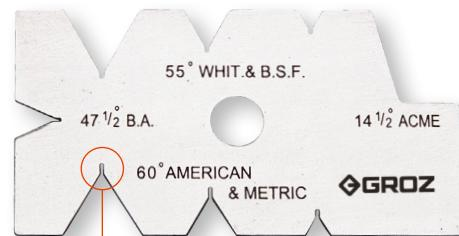
The gauge clearly indicates 55° for Whitworth and BSF Threads; 47-1/2° for BA Threads, 60° for Metric and American National Threads and 14-1/2° for Acme threads
